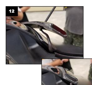
Adjust the slack in the wiring, make sure the wire is exiting the side area of the fairing. Using the provided remaining washers and the two 1/4-20 x 7/8 Allen head Bolts, install onto the fairing. Make sure the windshield trim is sitting on top of the wiring and that there is no wire slack remaining. Once the screws are started, make any final adjustments to fitment, then tighten all 3 top bolts.
