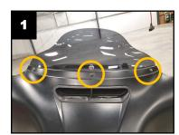
Remove the 2 T27 Torx bolts from the left bottom side of the inner fairing as shown. Save for reinstallation later.
