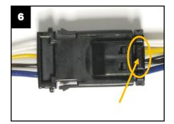
Unplug the connector by pushing in on the tab located on the male side of the connection, highlighted in the photo. Push the tab and pull apart both sides at the same time. Remove the turn signal assembly from the bike completely and store in a safe place for reinstallation shortly.
