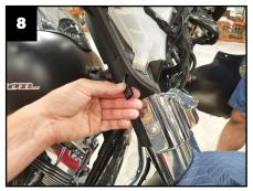
Push the Pass-through harness into the hole in the fork. Make sure that the Connector for the turn signal does not go into the hole. Plug the connector from the turn signal into the Pass-through harness, then reinstall the turn signal onto the fork frame and secure with the original nuts. Repeat for the other side.
