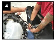
Remove the 1/2" nuts that secure the turn signal housing to the fork. Store in a safe place for reinstallation later. Pull assembly away from the fork to reveal the black wiring connector.
