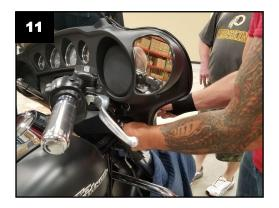
Reinstall the T27 Torx bolts into the inner fairing, make sure the longer bolt is in the top slot. DO NOT tighten down yet, we want to be able to adjust fitment of the wires and windshield trim.
