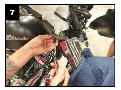
Plug the male end of the pass-through into the exposed female turn signal connector. Be sure the connector fully seats allowing the locking pin to snap in place. Repeat steps 5, 6 and 7 on the left side turn signal.
